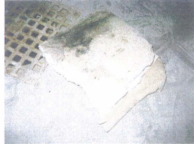
MCI – Kansas City Cable Access Level Mold Contaminated Drywall Scrap (Removed and Discarded During Survey)
